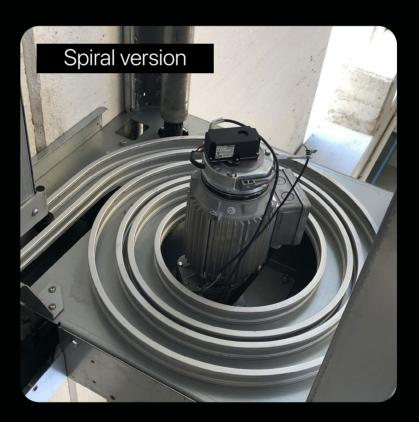
The spiral winding system allows a high thermal-acoustic insulation and an even smaller footprint.
